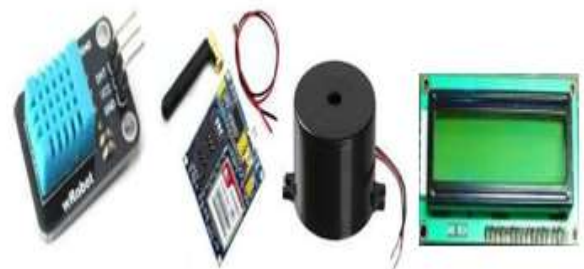
Figure2. DH-11 sensor, Buzzer, GSM modem (Sim900), Liquid crystal display unit (LCD)
